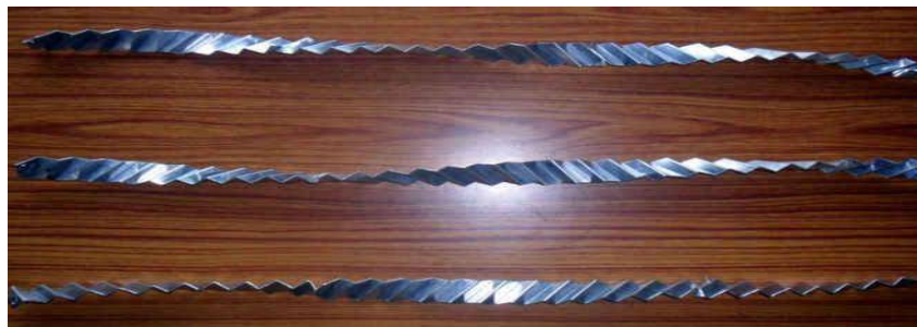
Fig 8 (a) Corrugated twisted tape insert
