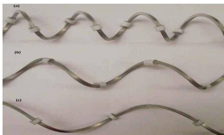
Fig 6 (a) The coiled-wire inserts with Teflon rings (a) P/D = 1 , (b) P/D = 2 , (c) P/D = 3 .
