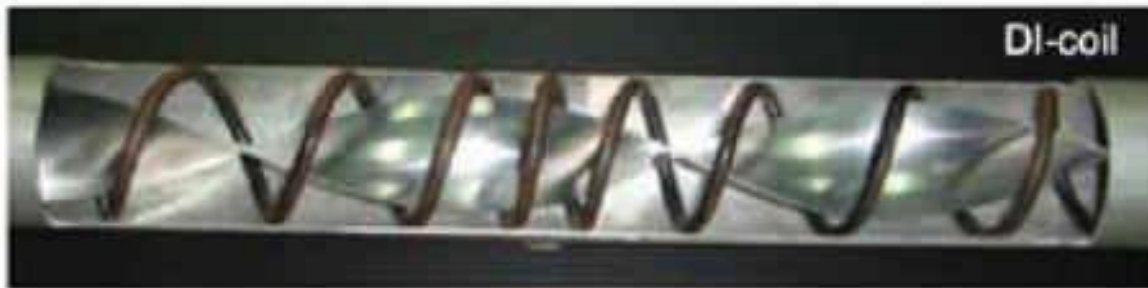
Fig 7 (c) The Test section fitted with wire coil and twisted tape
